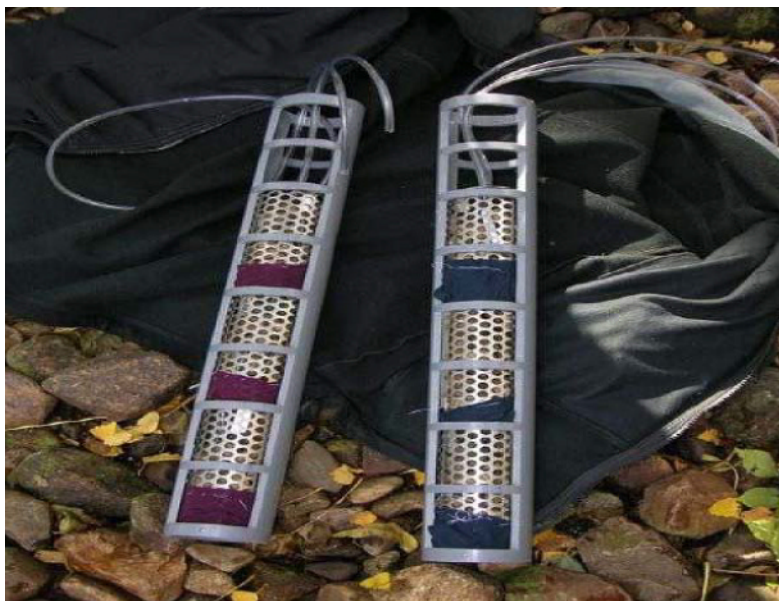
a) Colonization chambers comprising three stacked 15 cm long gravel-filled sub-chambers with tubing for extraction of water (Photo: Jane Grant)
