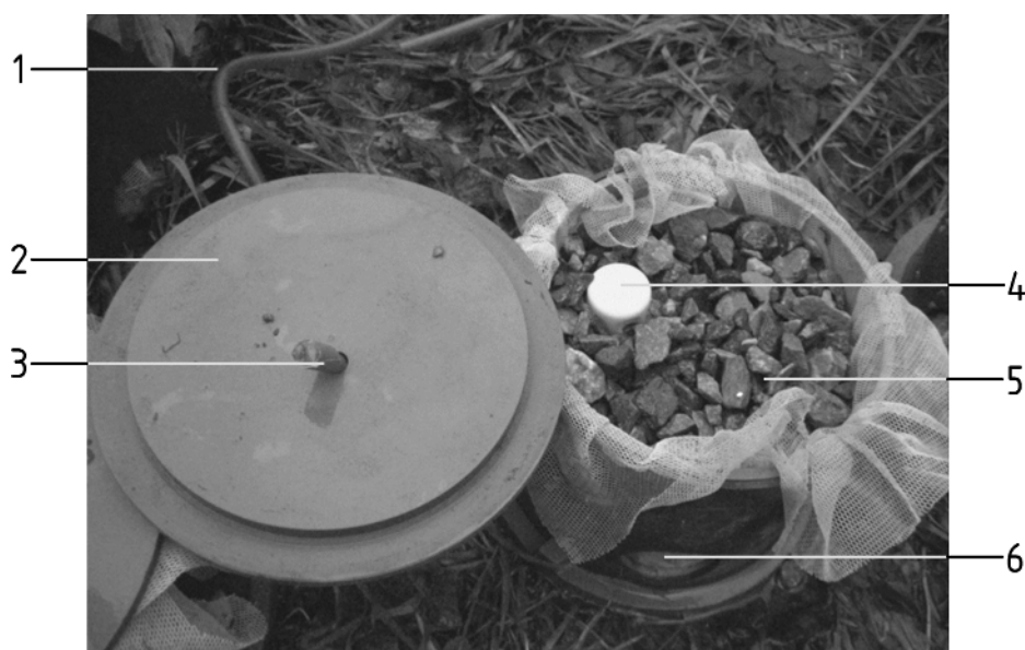
a) Colonization chambers comprising three stacked 15 cm long gravel-filled sub-chambers with tubing for extraction of water (Photo: Jane Grant)
