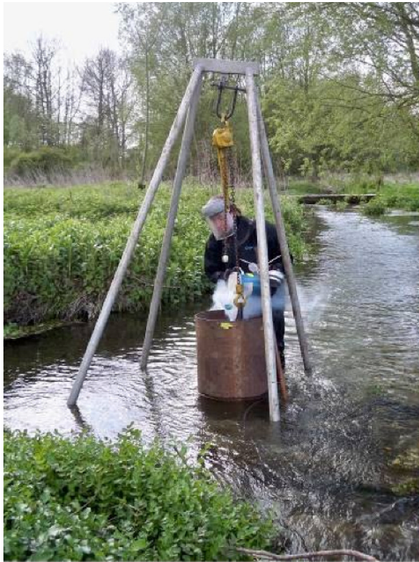
a) Frozen core being extracted
