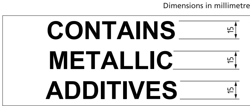
Figure NB.2 — Form of marking for automotive diesel with Biodiesel (B10) containing metallic additives
