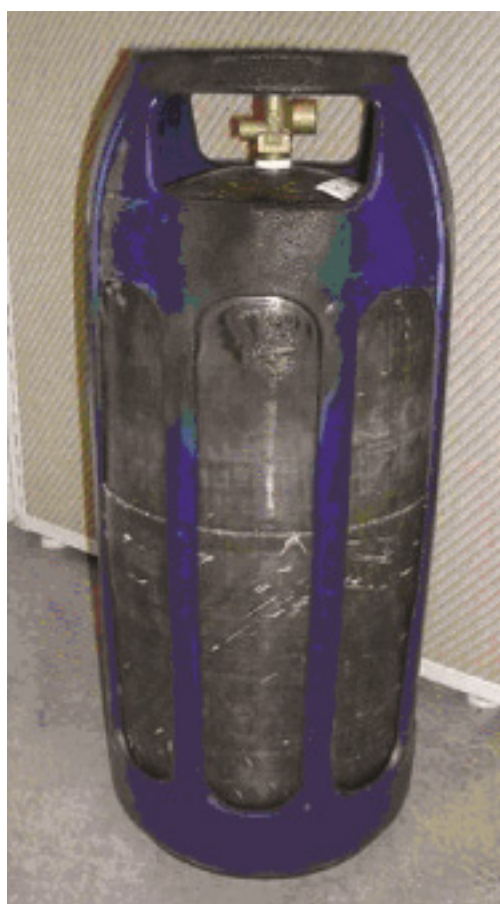
Figure C.6 — Heat and fire damage
