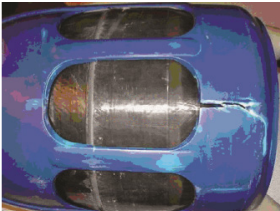
Figure C.5 — Defect protective casing: Broken casing
