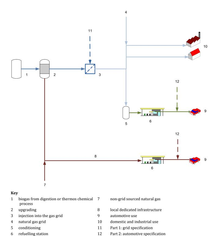
Figure 1 — Representation of some flows and uses of biomethane and natural gas
