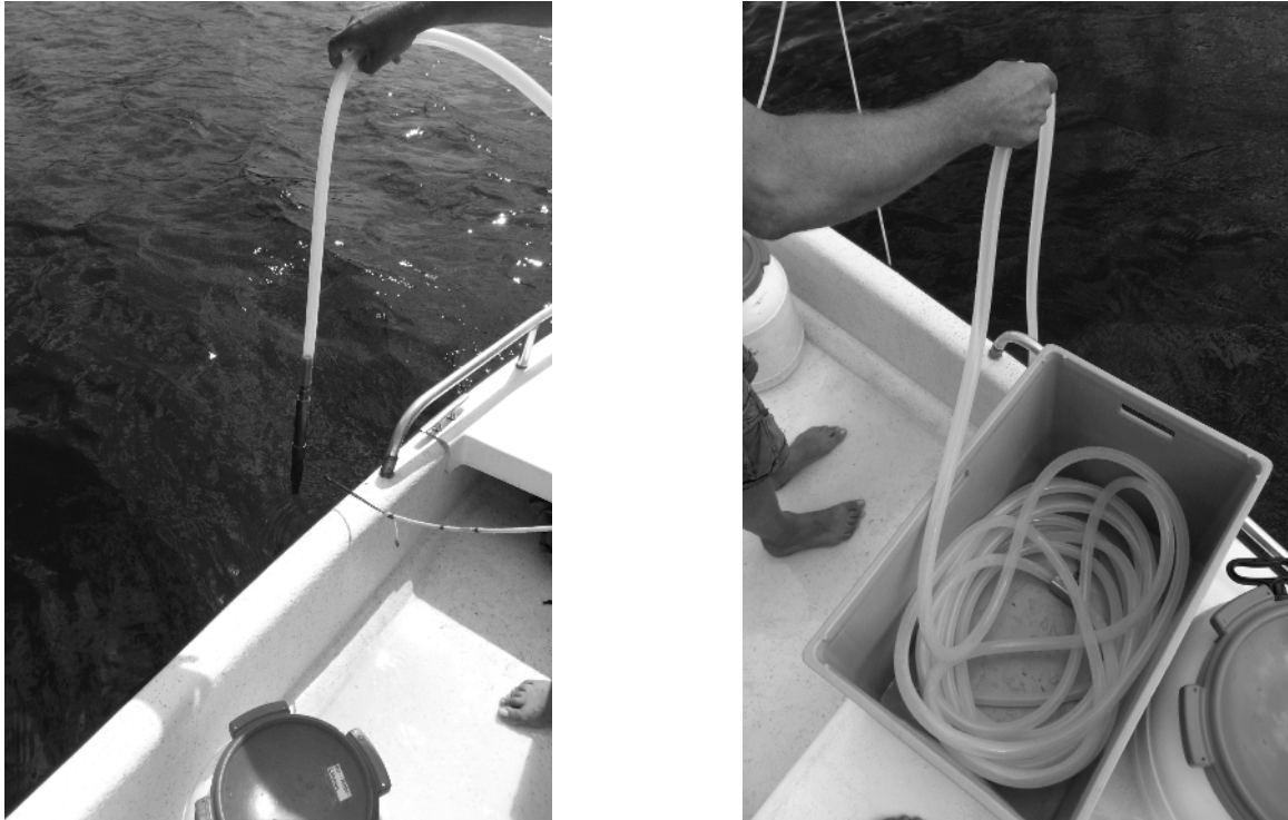
Figure B.3 —Integrating sampling using a hose developed by Brandenburg University of Technology Cottbus-Senftenberg, Germany (Photos ©Hoehn, LBH, Germany)
