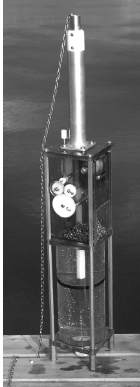
Figure B.6 — Mechanic integrating water sampler (Photo ©Uwitec Mondsee, Austria)
