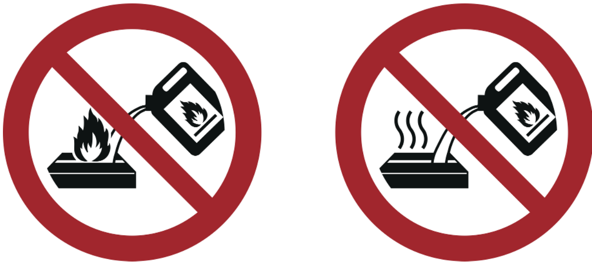
Figure 5 — Graphical symbols “Do not fill fuel into the open flame. Do not fill fuel into the hot burner”
