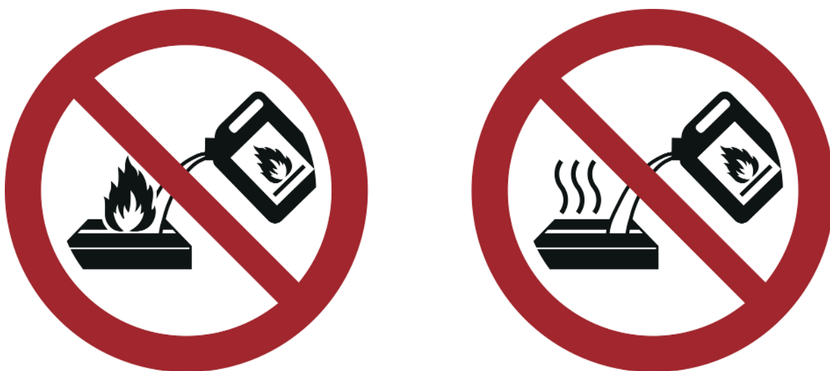
Figure A.1 — Do not fill fuel into the open flame. Do not fill fuel into the hot burner
