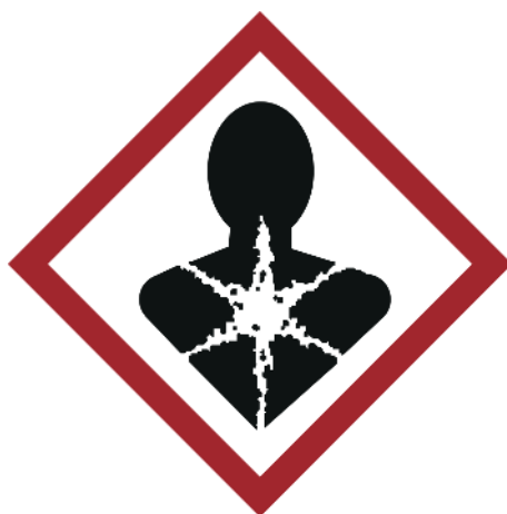
Figure A.10 — Health hazard
