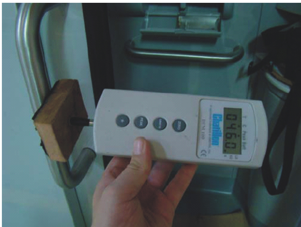
Figure C.1 — Example of a force meter being used to measure the force required to push a sliding door
