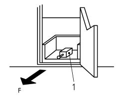
b) friction test piece shown on internal step for access or egress to the vehicle
