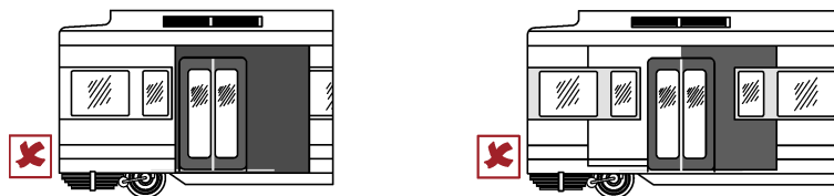
Figure B.8 — Non-compliant examples as the contrasting area is not centred on the axis of the door
