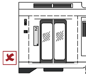
Figure B.5 — Example of where the window is greater than 40 % of the total visible area of the door leaf
