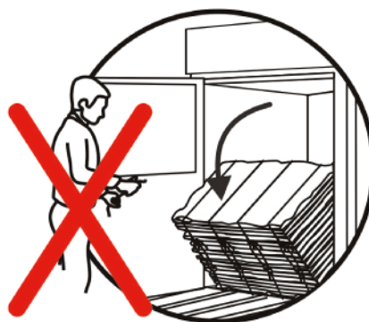
Figure 3 — Warning sign against standing in front of the unloading opening
