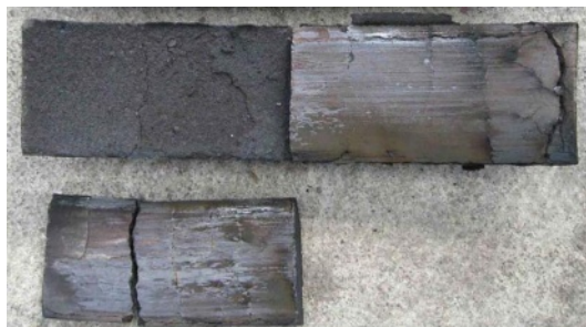
Figure U.6 — Detachment of the friction material
