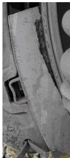
Figure U.2 — Crumbling of the friction material
