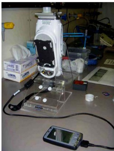
Figure A.3 — Measurement of a sample collected in a cup – Hand-held instrument mounted on a stand
