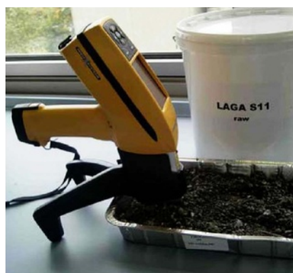
Figure A.2 — Direct measurement – Hand-held instrument mounted on a stand
