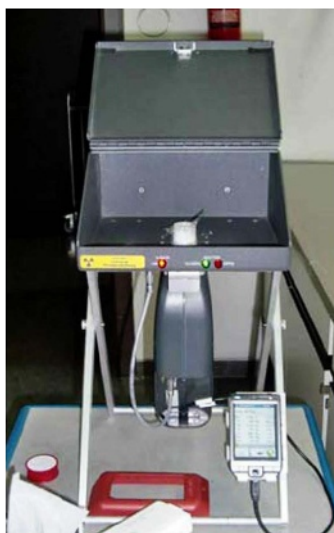
Figure A.4 — Measurement of a sample collected in a cup – Hand-held instrument mounted on a stand – Using a radiation shield
