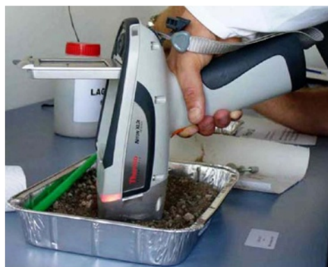
Figure A.1 — Direct measurement – Hand-held setup
