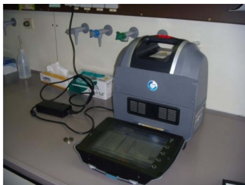
Figure A.5 — Compact bench top XRF spectrometer
