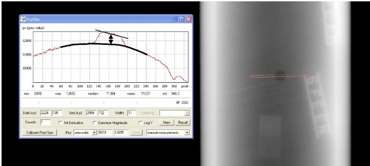
Figure B.2 — CR image of a 3” test pipe containing internal holes and showing a step wedge for calibration of the attenuation coefficient
