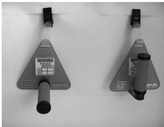
Figure B.2 — Radial sampler supporting plate
