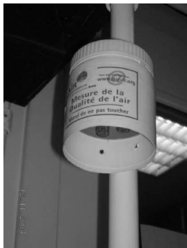
Figure A.3 — Tube type sampler with a cylindrical tube with shelter
