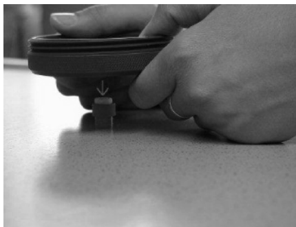
Figure A.7 — Glass frit membrane inserted into the sampler end cap
