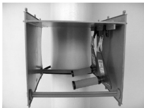
Figure B.3 — Radial sampler shelter
