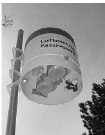
Figure A.6 — Tube-type sampler with shelter
