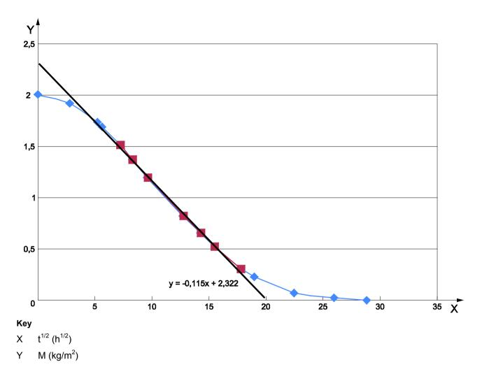
Figure A.2 — The drying rate, corresponding to the second drying phase, is therefore  $D_2 = 0.115 \text{ kg/m}^2 h^{1/2}$
