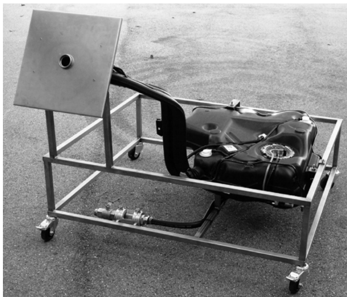
Figure 2 — Example of a test tank from VW Golf according to Annex A mounted in a frame and fitted with a plate simulating the motor vehicle body in close proximity to the tank filler neck
