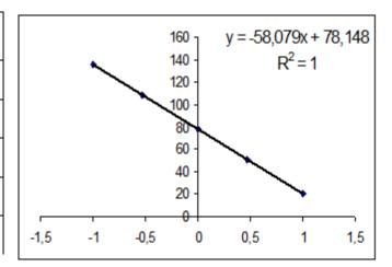
Figure 1 — Example of plotting of the electrical potential Y in (mV) of the fluoride concentration X in (mg/l) of the calibration standards (8.2) as a function of the logarithm (= Log [X]) and determination of the slope (e.g. 58,079) in the linear region of the calibration function
