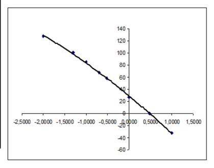
Figure C.1. — Example of plotting of the electrical potential Y in (mV) of the fluoride concentration X in (mg/l) of the calibration standards (8.2) as a function of the logarithm (= Log [X]) for interpolation reading in the non-linear region of the calibration function
