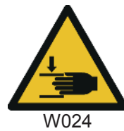
Figure 7 — Sign trapping and crushing hazard
