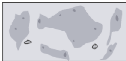
Figure A.3 — CODE T2 - Oxidation only around minerals without runs of oxidations
