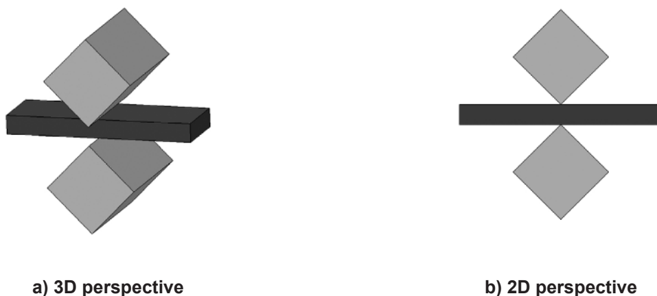
Figure C.1 — Principle of wedge penetration test
