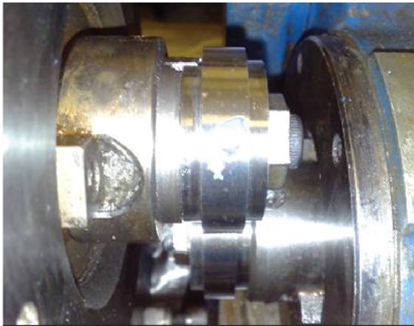
Figure L.2 — Simulated wheel/rail contact using a wheel and rail disc(s)
