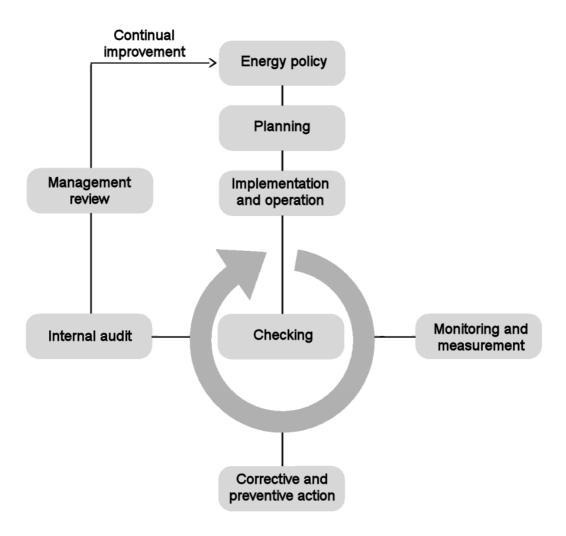
Figure 1 — Energy management system model for this standard
