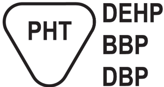
Figure A.7 — Example of the symbol for "CONTAINS OR PRESENCE OF PHTHALATE"
