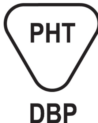
Figure A.4 — Example of the symbol for "CONTAINS OR PRESENCE OF PHTHALATE"
