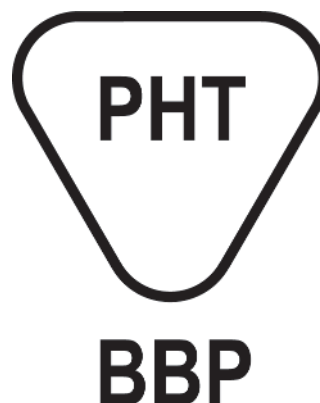
Figure A.6 — Example of the symbol for "CONTAINS OR PRESENCE OF PHTHALATE"
