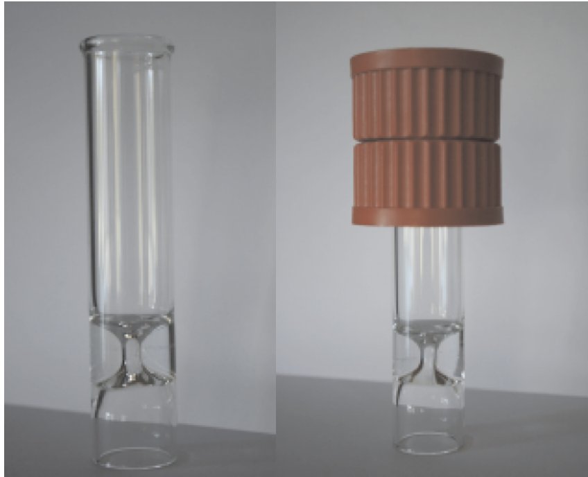
Figure A.4 — Glass liner (left) and glass liner within the screw caps (right)
