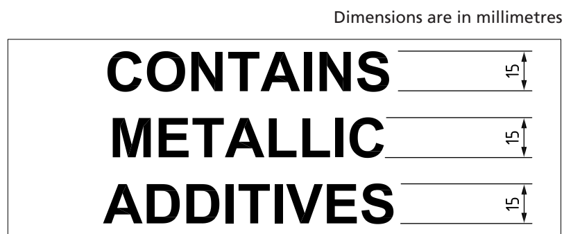
Figure NB.2 — Form of marking for paraffinic diesel fuel containing metallic additives
