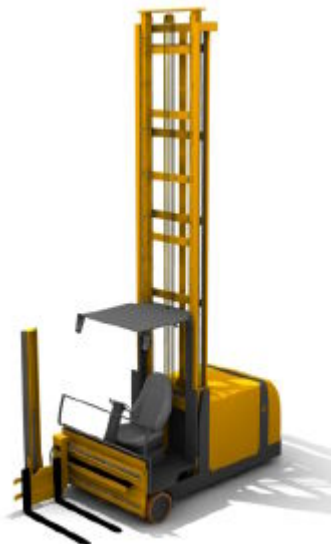
Figure A.8 — Very narrow aisle trilateral man-down pallet truck with rotating fork
