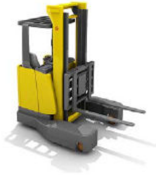
Figure A.10 — Four way truck
