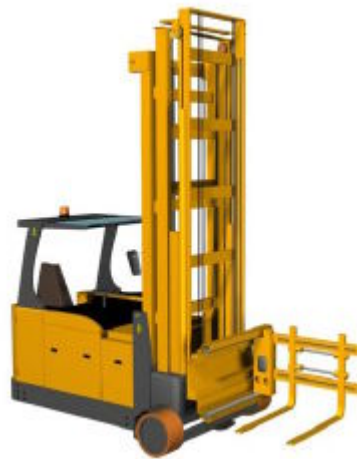
Figure A.8 — Very narrow aisle trilateral man-down pallet truck with rotating fork
