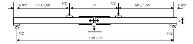
Figure 1 — Test arrangement for measuring the local withdrawal in bending
