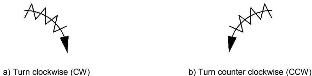
Figure 2 — Fail safe directions for part-turn actuators
