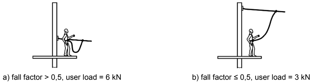
Figure 4 — Fall factors and user loads for single ropes zip lines
