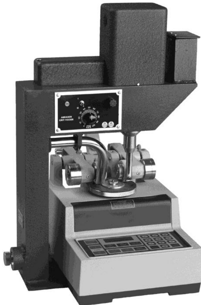
Figure A.3 — Example of a Taber Abrader with Grit Feeder
