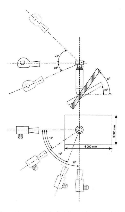
Figure 7 — Test rig for type C boilers fitted with a vertical terminal on a pitched roof
