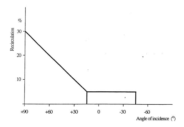
Figure N.1 — Maximum permitted recirculation of the combustion products
