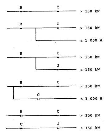
Figure H.2 — Heat inputs up to 300 kW
