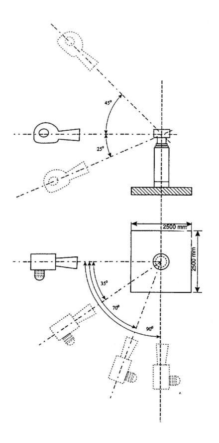
Figure 6 — Test rig for type C boilers fitted with a vertical terminal on a flat roof
