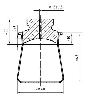
Figure 1 — Example of a capillary-stoppered pyknometer
