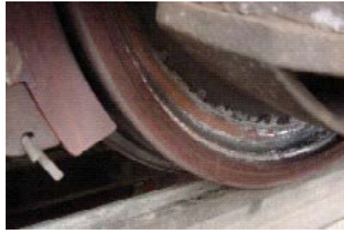
Figure C.32 — Overheating of the rim/web transition zone
