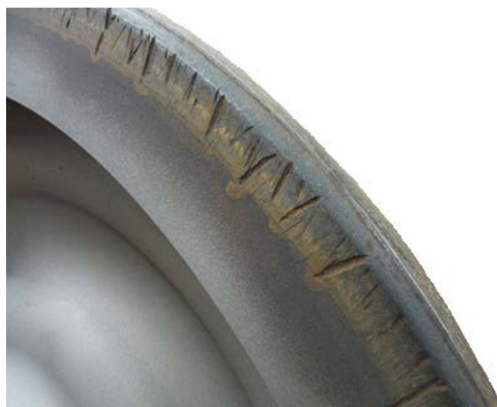
b) Radial defects on the internal side of the rim
