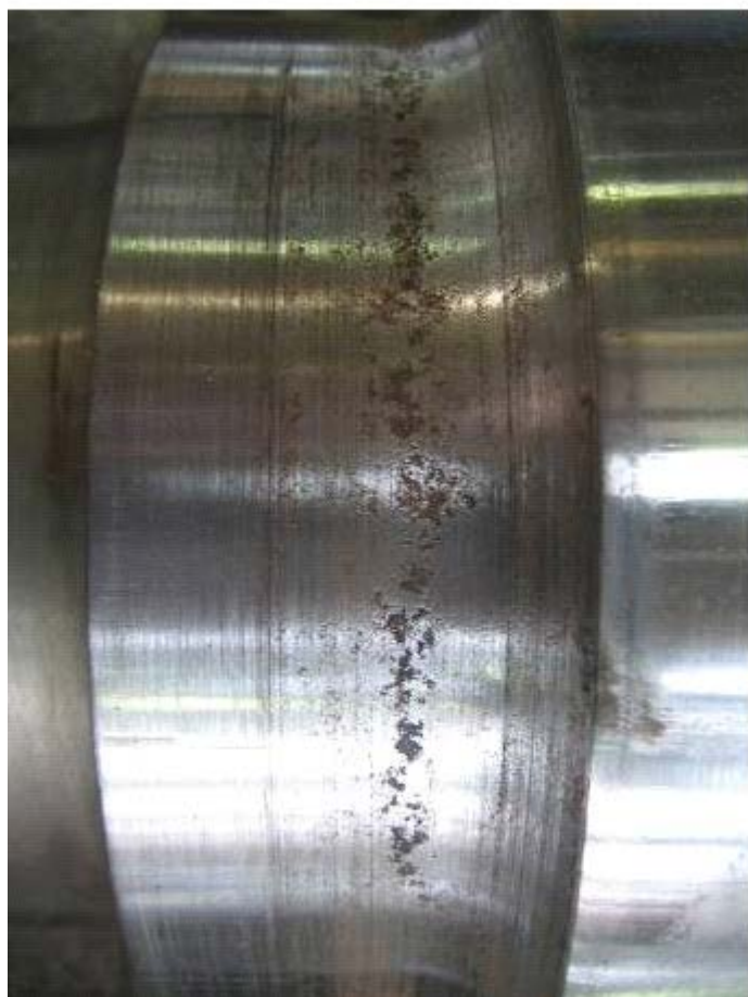
Figure I.3 — Corrosion defects in abutment area and transition radii
