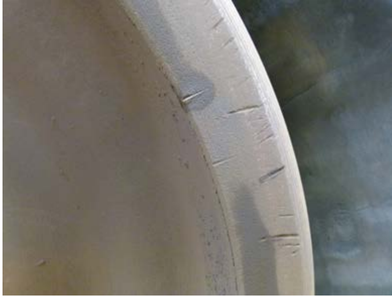
c) Radial defects in the rim/wheel plate transition
