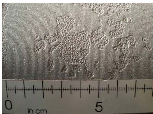
Figure I.1 — Localized and severe defects on the axle surface
