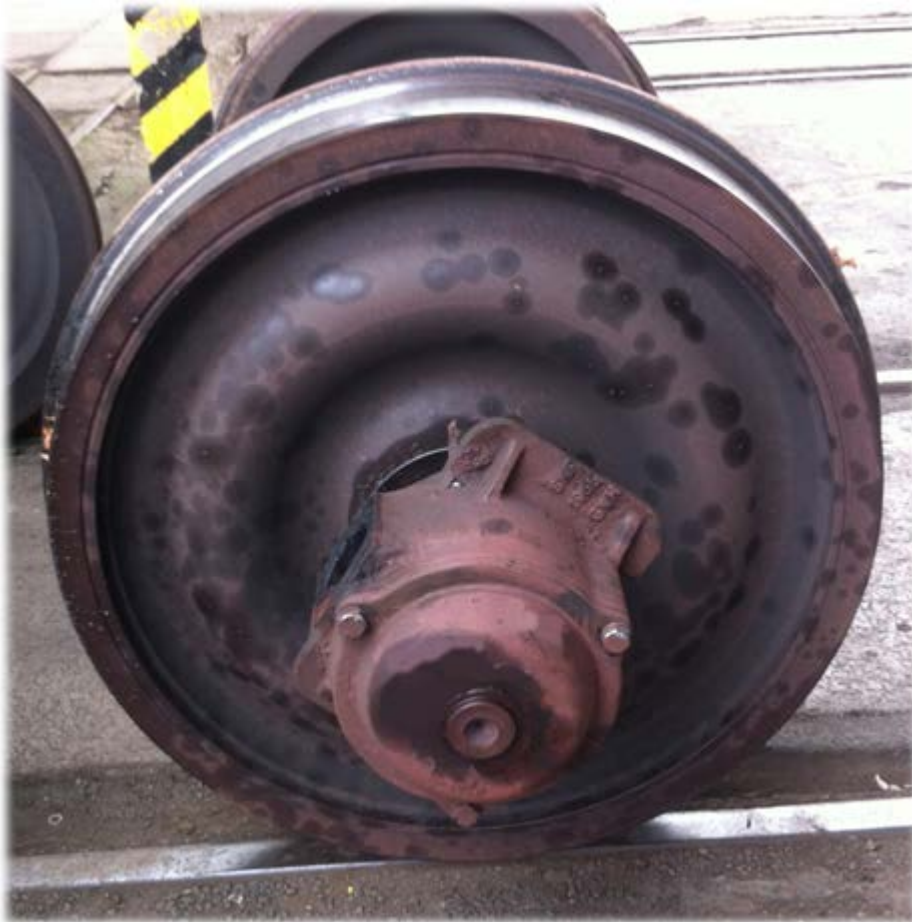
Figure C.41 — Traces of lost grease/oil projected onto the wheel plate
