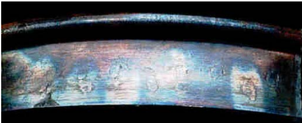
Figure C.33 — Overheating of the tyre
