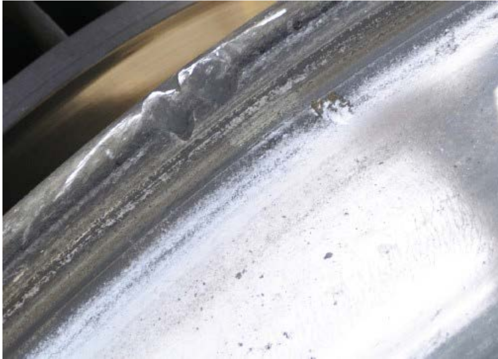
Figure C.21 — Damage on the flange
