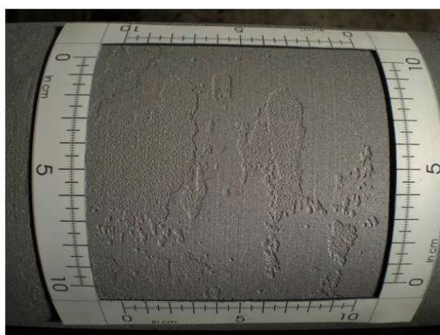
Figure I.1 — Localized and severe defects on the axle surface
