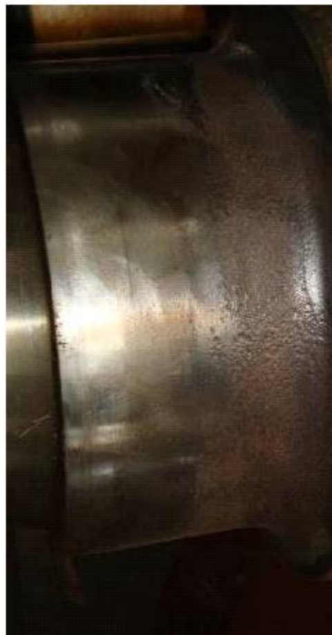
Figure I.3 — Corrosion defects in abutment area and transition radii
