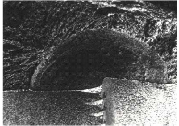
b) Evolution of a fatigue crack initiated from a lathe driving tool mark
