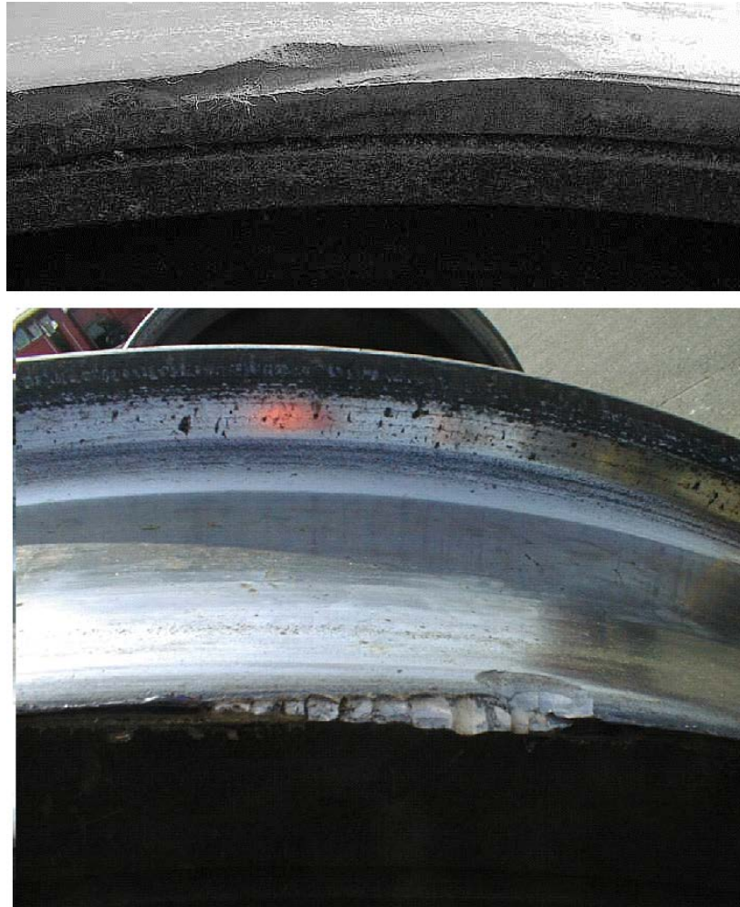
Figure C.16 — Damage to the chamfered corner
