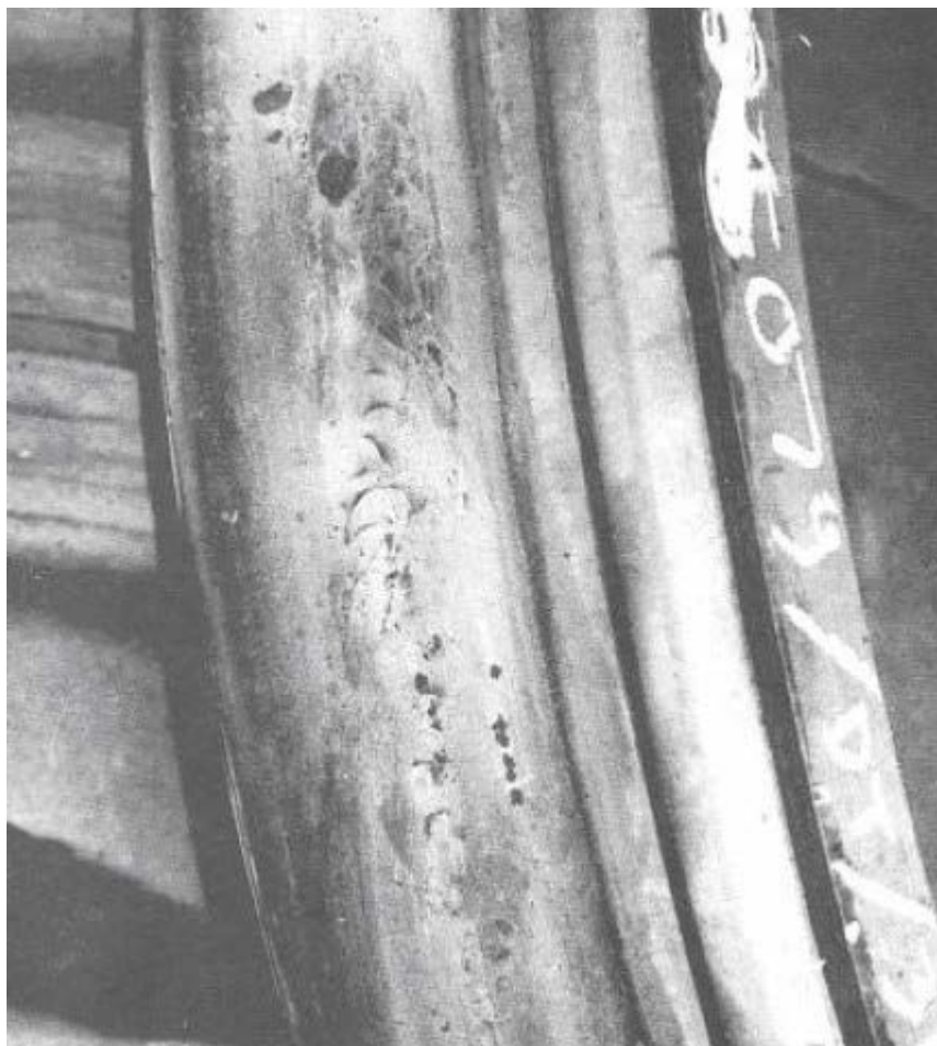
Figure C.2 — Multiple wheel flat
