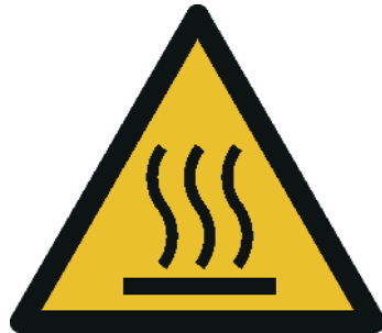
Figure 13 — Warning sign “Caution, hot surface”
