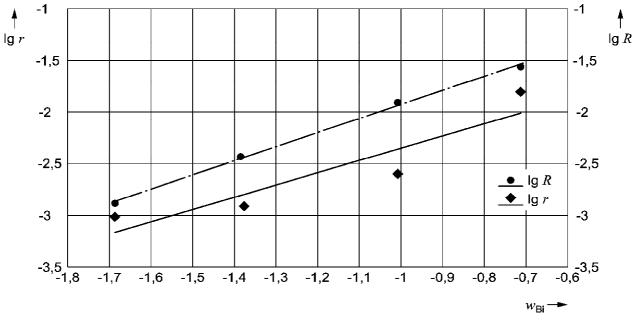
**Key**  $\lg r = 1,180 \text{ 1 } \lg w_{\text{Bi}} - 1,170 \text{ 6}$   $\lg R = 1,361 \lg w_{\text{Bi}} - 0,566 \text{ 9}$
