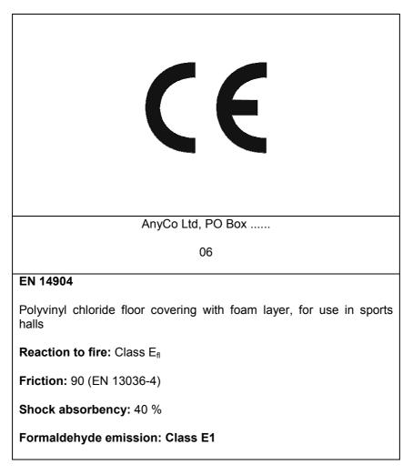
Figure ZA.1 – Example of CE marking for product classified in reaction to fire Class Eff
