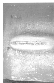
Figure C.4 — Arc or torch burns
