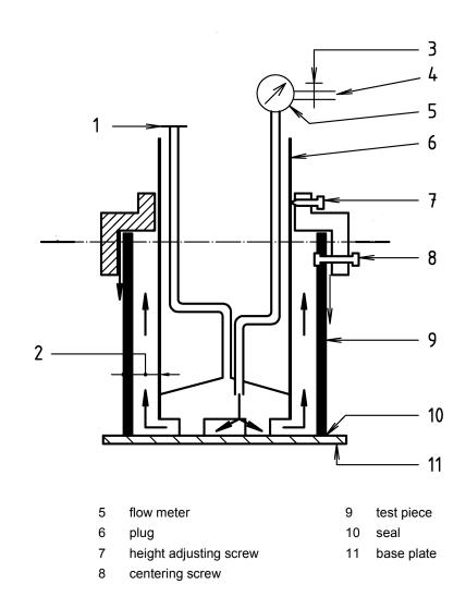
Figure B.1 - Example of an arrangement for flushing large diameter pipes, side view
