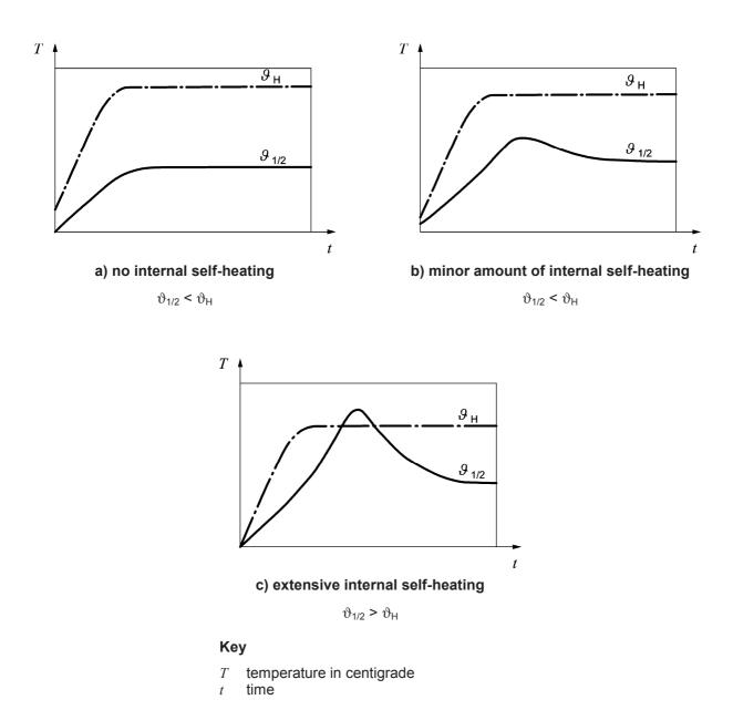
Figure A.1 — Typical temperature profiles during the test for the internal self-heating versus time
