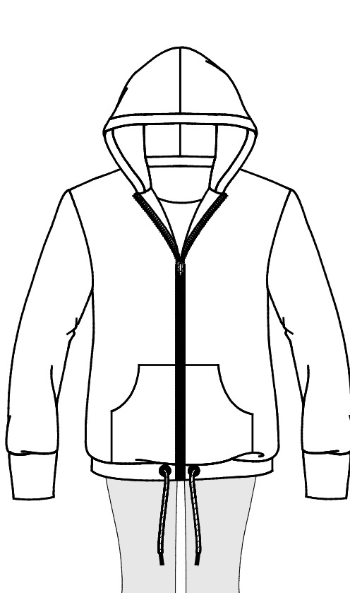
Figure F.13 — Example of unacceptable cords at lower edge of garments hanging below the crotch (see 3.5.1)
