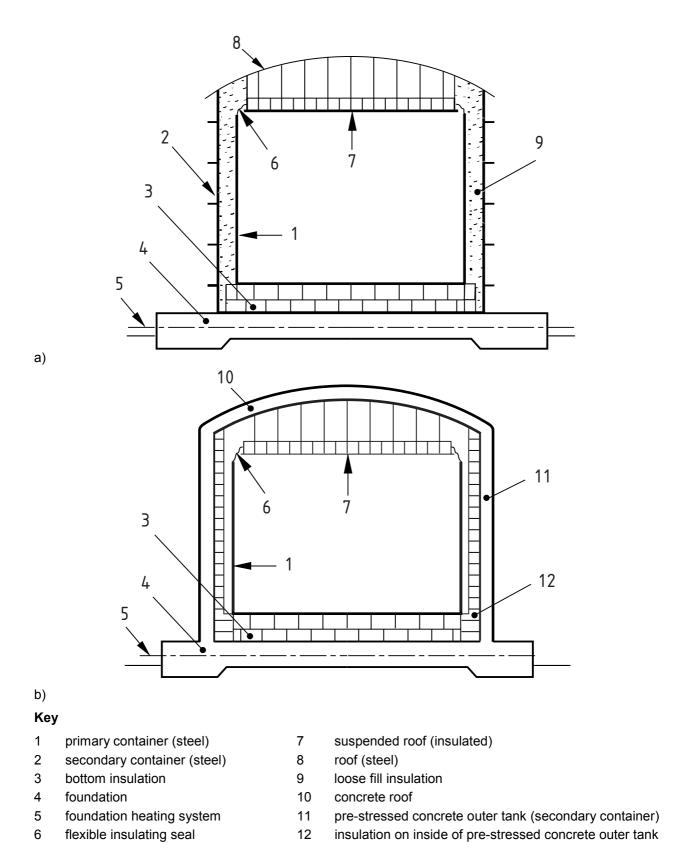
Figure 3 — Examples of full containment tanks
