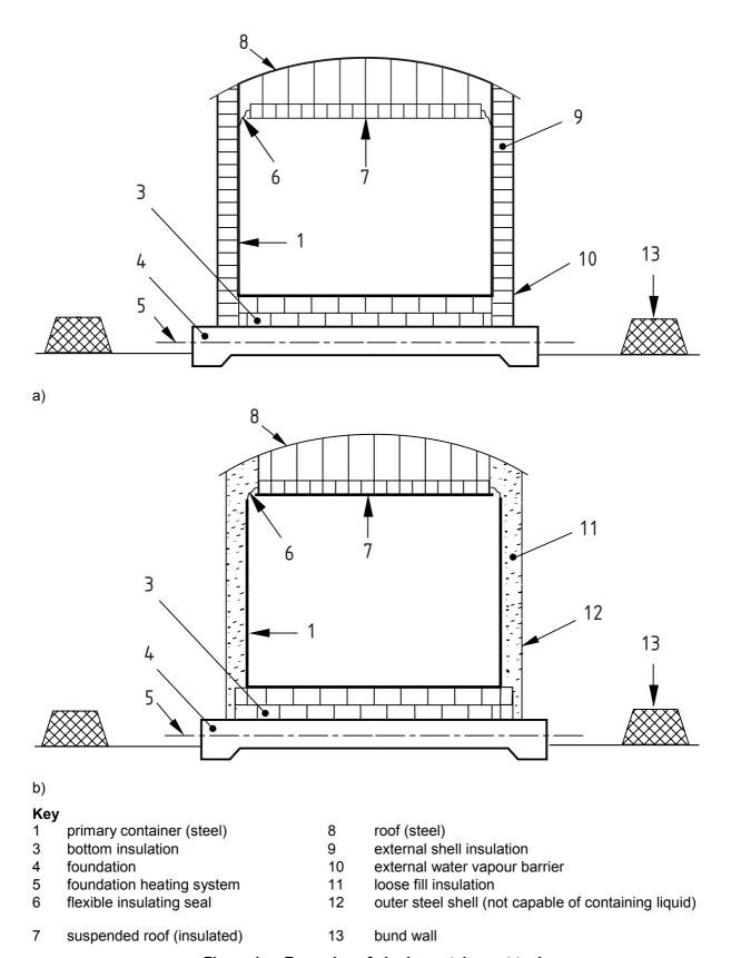
Figure 1 — Examples of single containment tanks
