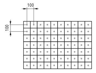
Figure 5 — View of test hearth and walls showing position of measurement points
