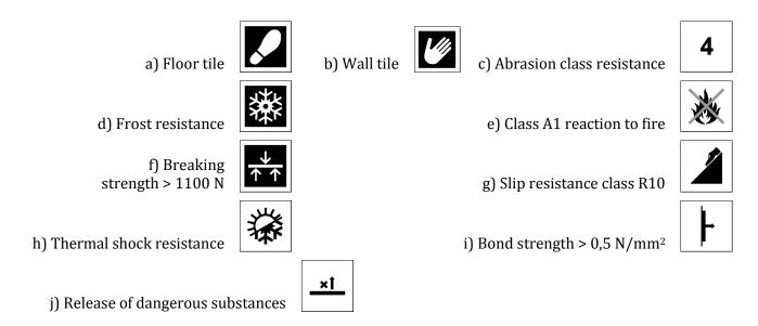
Figure P.1 — Examples of symbols of indication of the intended uses and of the names and performances of some characteristics of ceramic tiles
