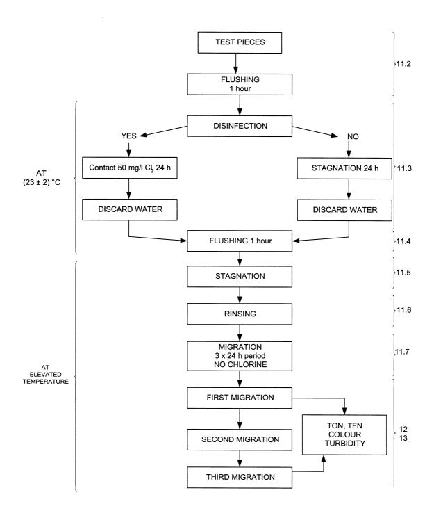
Figure A.2 — Products to be tested at elevated temperatures
