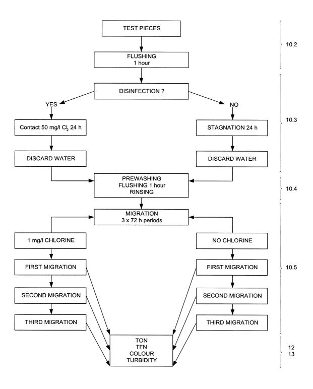
Figure A.1 — Products to be tested at  $(23 \pm 2)$  °C
