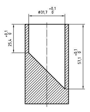
Figure 4 — Small parts cylinder
