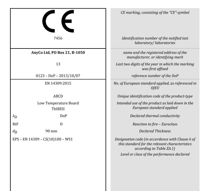
Figure ZA.1 — Example CE marking information of products under AVCP system 3
