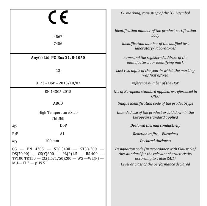
Figure ZA.1 — Example CE marking information of products under AVCP systems 1 and 3
