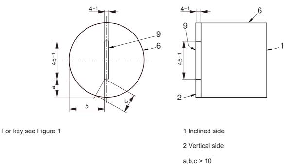
Figure 2 — Position of the slot at the base of the flow guidance hopper in case of cylindrical cross section (left) and of rectangular cross section (right)
