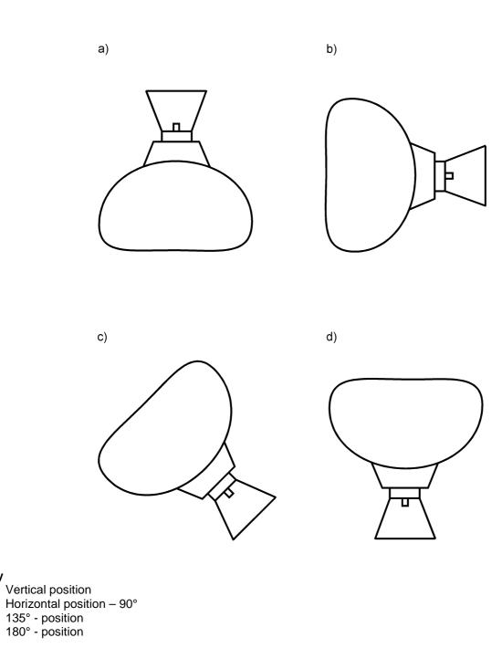
Figure A.3 — Leakage test
