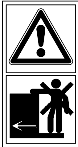
Figure B.3 — Ascending onto the machine while operating is dangerous
